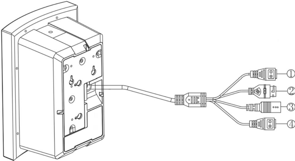
① Amplifier output connector: connector color is black, specification is 3.81-2P, connecting external speaker, when the speaker receives the broadcasting, the same sound can be heard from the speaker. The Rated impedance:8Ω,the rated output power:30W
